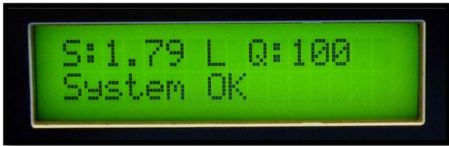
Figure 6-1: Normal Mode showing Good Signal
